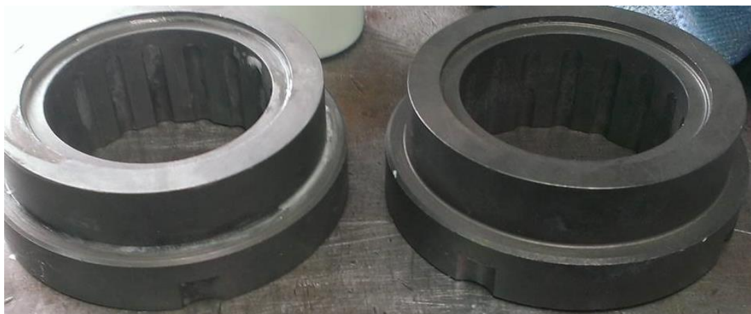
Mould cleaned with Blu 1000 and coated with 640. (Left side) Used for moulding vulcanised auto parts (Italy).
