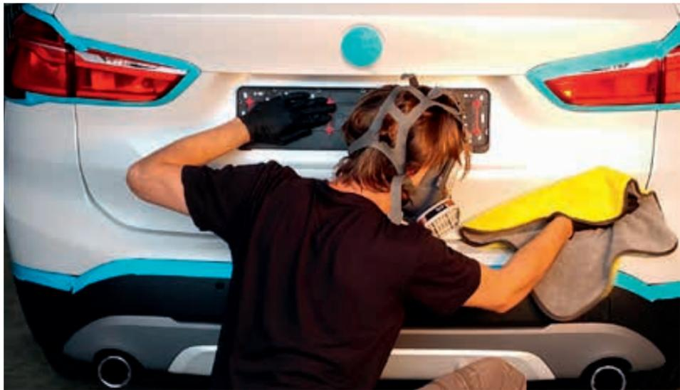
The coating will cure faster if the surface is hot and so it will be advantageous to place the car in direct sunlight after the first 2 hours of curing.
