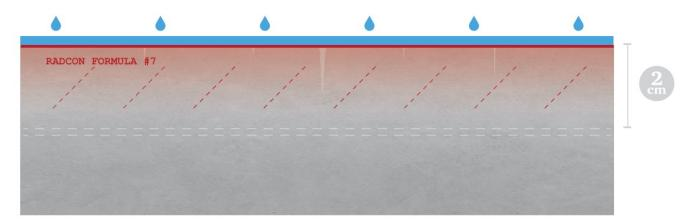
Concrete surfaces treated with Radcon Formula  $\#7^{\$}$  with cracks from 0.2 to 2 mm are 100% waterproof. The cracks will be completely slowly closed by the expansion of Radcon Formula  $\#7^{\$}$ .
