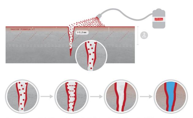
Concrete surface with hairline cracks treated with Radcon Formula #7 remains 100% waterproof. The cracks will be completely closed by the expansion of Radcon Formula #7<sup>®</sup>.
