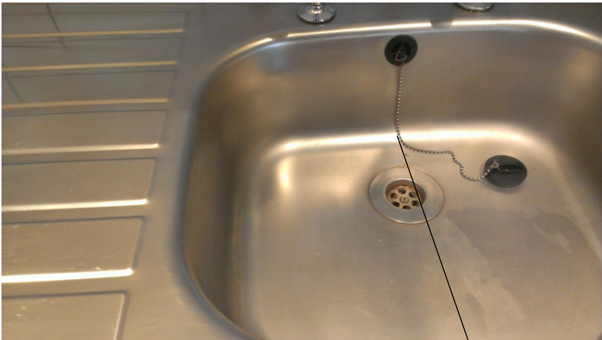
Cleaned with Stainless Steel Cleaner BLU1000 and coated with Universal 675. It was noted that there was already a coating in place on the sink. This will inhibit bonding of SiO 2 layer.
