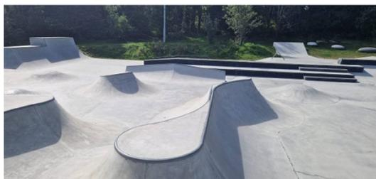
This well used Skate-park had to be cleaned prior to being sealed with a protective layer. The local council stressed that a completely environmentally friendly cleaner should be used. Biosativa® was spray applied at 1:20. The surface was then rinsed with a "light" pressure washer. The newly cleaned surface not only looks like new but cleaning with Biosativa® has resulted in the removal of oils and sugars, (from soft drinks).
