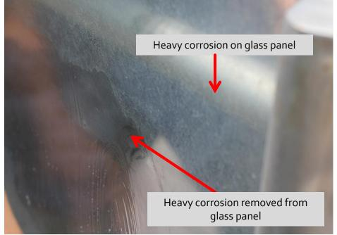
Removing Glass corrosion like watermarks, scaling and grime from corrosion is very difficult or sometimes impossible.
