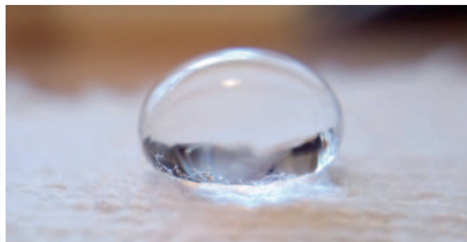
Fabrics coated with HNSFT technology after 15 wash cycles.
