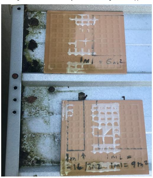
The 7620 penetrative coating was applied to the boxed area but as it is a penetrating coating it migrates. The level of migration is shown by the blue line. The area beyond the blue line is now saturated and mold is established within the stone. The coated area is completely dry and mold free.
