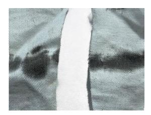
After one minute the oil has spread into the fabric
