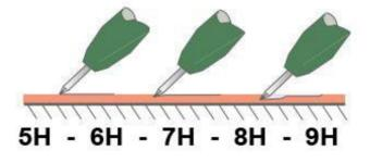
CCM Permanent Protector forms a layer hardness of **6H until 9H** depending to the coated substrate and the curing method.
