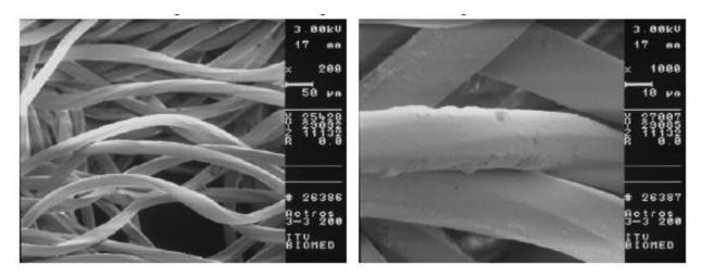
These images show fibres coated with Liquid Glass. You will note the spaces between the fibres. Liquids will pass through these gaps but the fibre is clearly protected against staining. Thicker "old tech" coatings will fill these gaps to produce a water proof but stiff and non-breathable coating.
